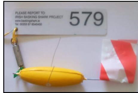
Five developed and tested MK 10 PATF Fastloc GPS Tags and a Timed Depth Recorder with visual tag ready for deployment
